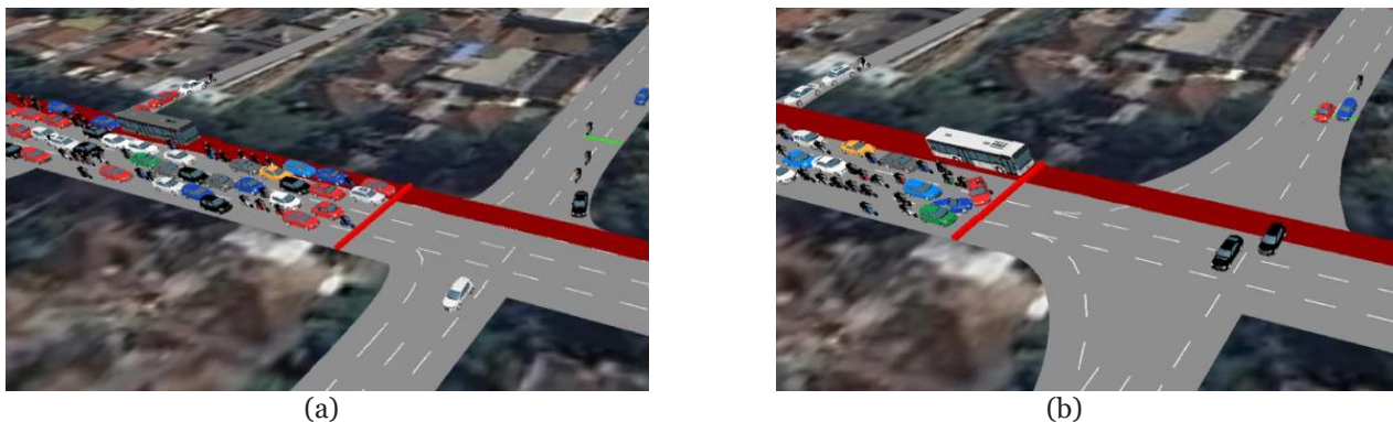
Fig 5. Illustration of the difference in conditions for BRT dedicated lanes: (a) without TSP and ATCS, (b) with TSP and ATCS
