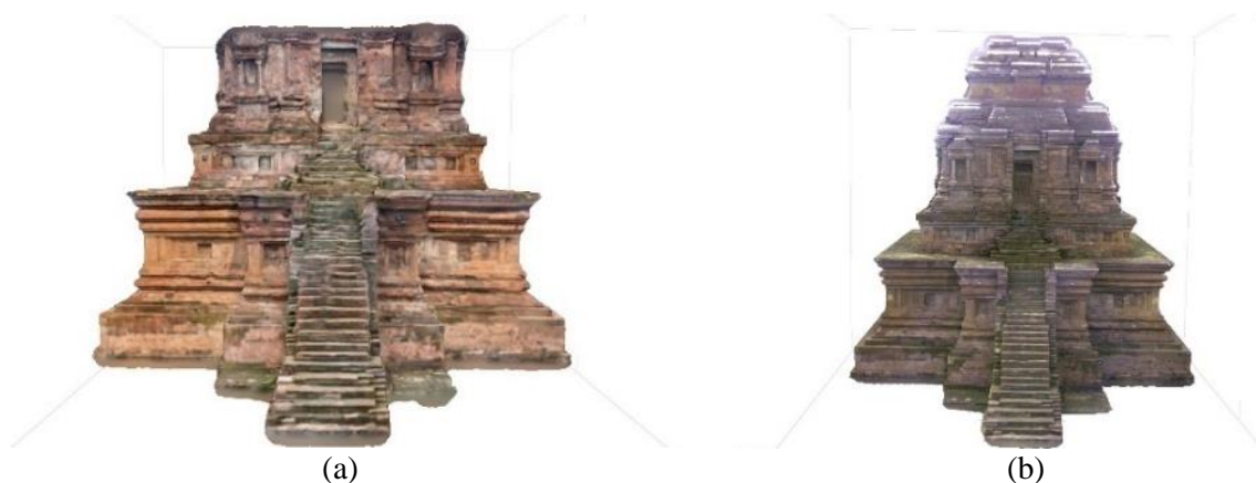
Gambar 7. Model 3D Bagian Depan Candi Gunung Gangsir (a) Low-Cost LiDAR (b) Terrestrial Laser Scanner
