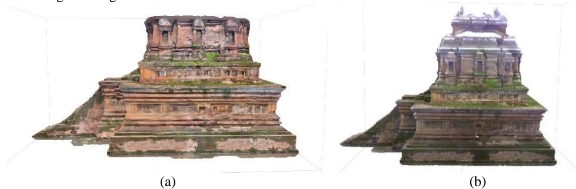
(a) (b) Gambar 8. Model 3D Bagian Kanan Candi Gunung Gangsir. (a) Low-Cost LiDAR (b) Terrestrial Laser Scanner
