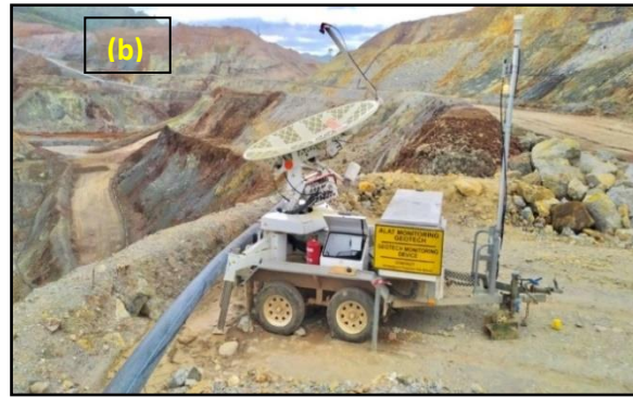
Figure 2. Pixel photo (a) and Slope Stability Radar (SSR605-XT) (b)
