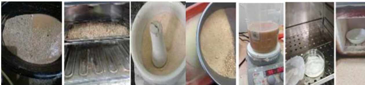
Figure 1. The fly ash was first dried and ground, then reacted with 3 M NaOH at 100 °C for 4 hours. The resulting mixture was subsequently precipitated using 6 M HCl and calcined at 800 °C for 3 hours. The obtained product was then further reacted with 6 M NaOH for 24 hours to produce sodium silicate
