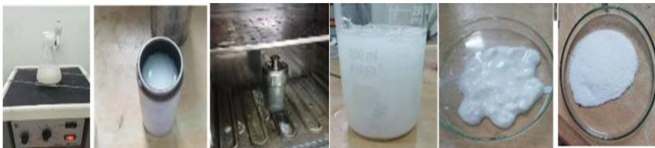
Figure 2. Silica–alumina catalysts were synthesized from fly ash-derived silica using a hydrothermal method through the reaction of sodium silicate and sodium aluminate at a 1:1 ratio in an autoclave at 100 °C for 3 days. The resulting mixture was then aged for 24 hours, followed by filtration, neutralization, and drying. The obtained solid product was identified as a silica–alumina catalyst.
