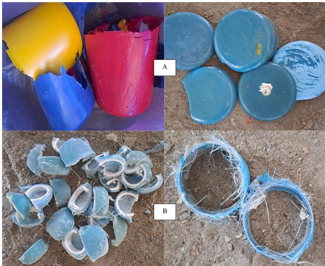
Figure 2. FRP composite waste in solid form: (a) pure, (b) impure
