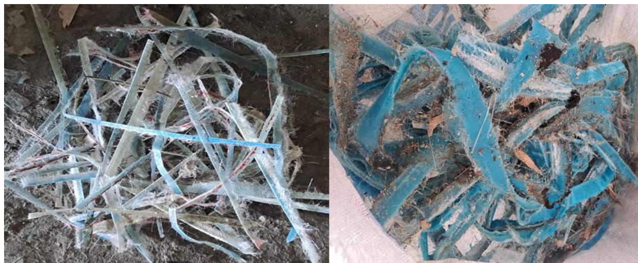
Figure 3. FRP composite waste in form of sheets/plate
