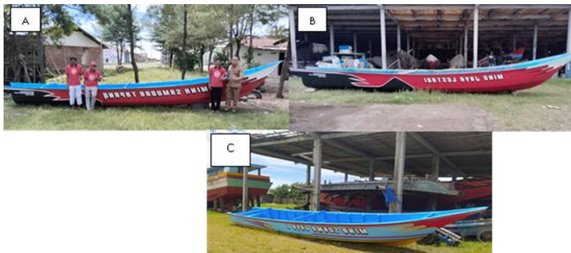
Figure 1. FRP vessels produced by CV. Roni Marine shipyard: (a) vessel with a size of 1,24 GT, (b) vessel with a size of 1,28 GT and (c) vessel with a size of 2 GT
