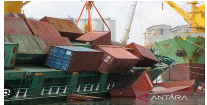
Figure 6. Lashing Container not Installed
