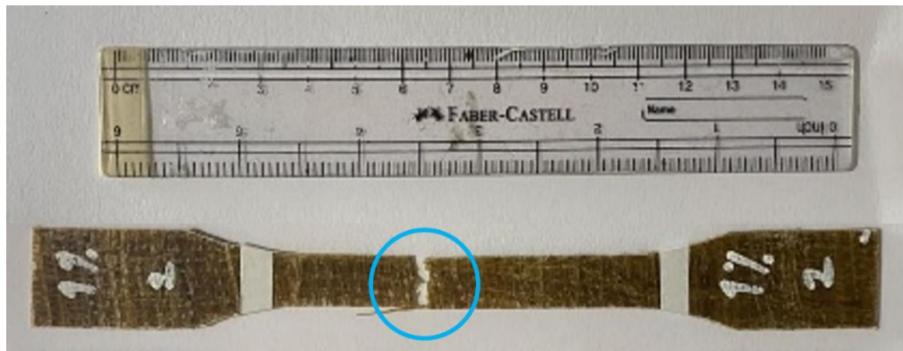
Figure 2. Tensile testing specimen
