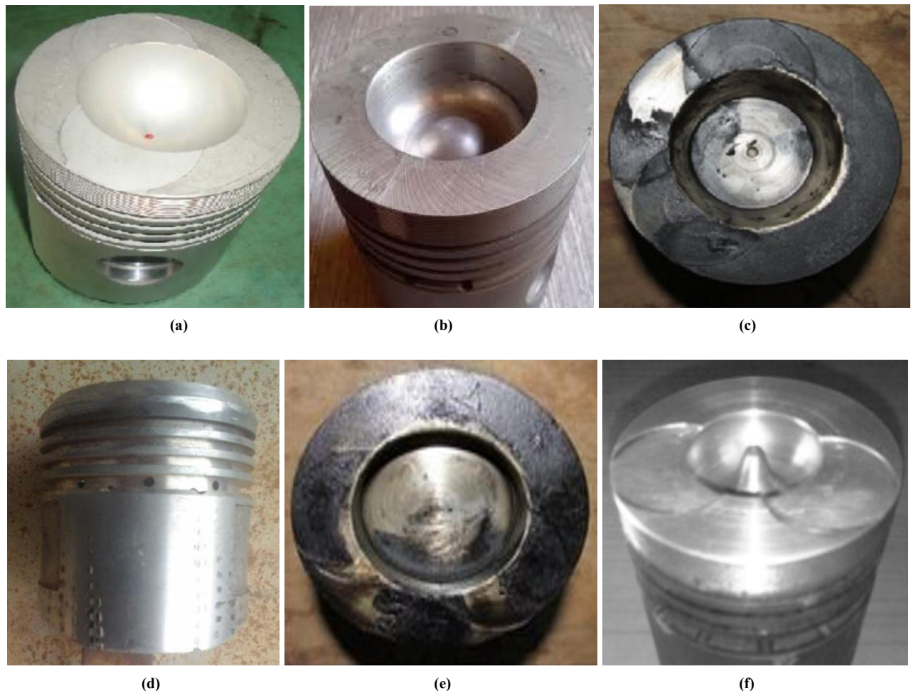
Figure 1. Several piston geometries a) hemispherical [22] b) toroidal [23] c) trapezoidal [24] d) truncated cone [25] e) cylindrical [24] f) re-entrant [26]
