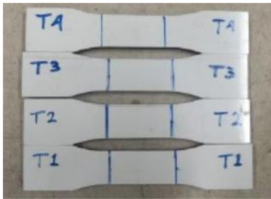
Figure 13. ICB standard test specimens
