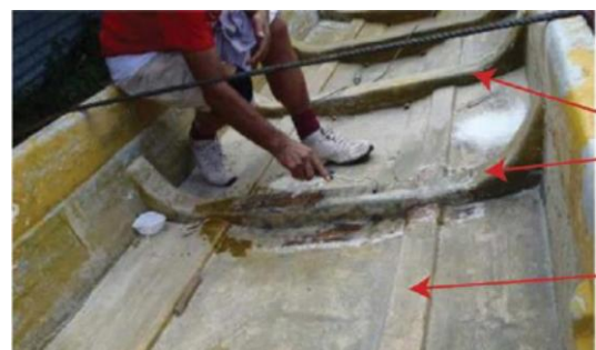
Figure 6. Frame and Louder Damage
