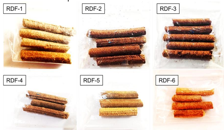
Figure 5. Visual appearance of RDF pellets under variation of biomass waste and CaO blend compositions.
