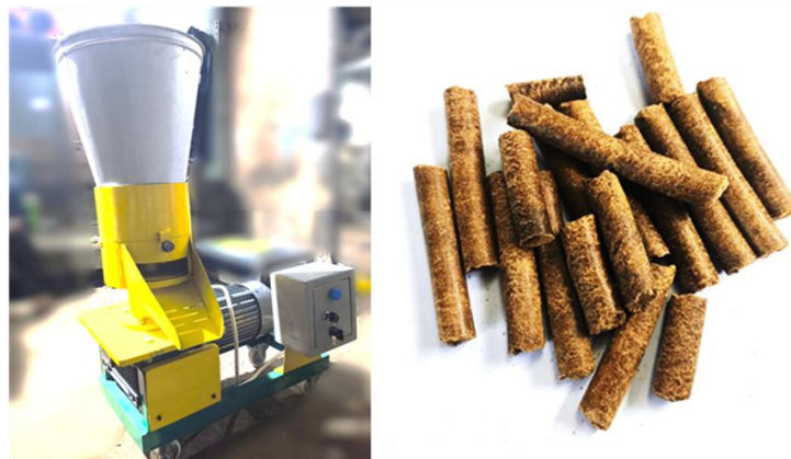
Figure. 2. Design of pelletizer machine for making RDF pellets. The pelletizer uses rollers to compress RDF material into uniform pellets (typically 6-10 mm diameter).
