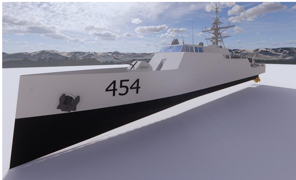
Figure. 12. 3D Visualization of the Selected Corvette Warship with Axe Bow Hull Form.
