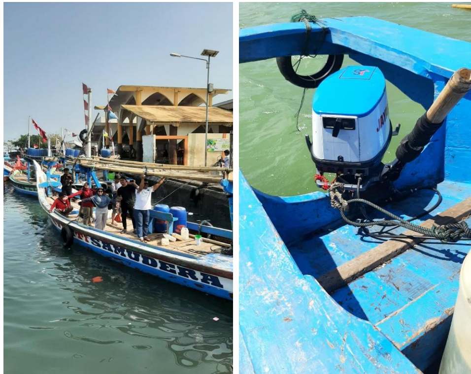
Figure 2. a) Seine net boat in Pelabuhan; b) Yamaha outboard engines with a power output of 40 HP.
