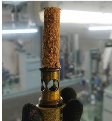
Figure. 3. Scale at Water Block Filter
