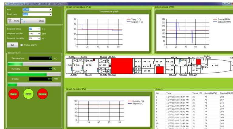
Figure. 11. Temperature and Smoke Sensor Test Results
