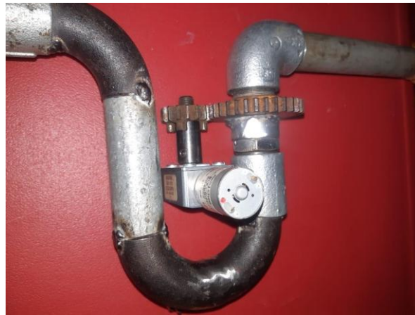
Figure. 6. Fire Nozzle Gear Construction
