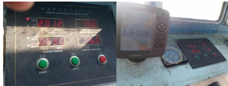
Figure 6. Engine RPM and GPS During the Sea Trials
