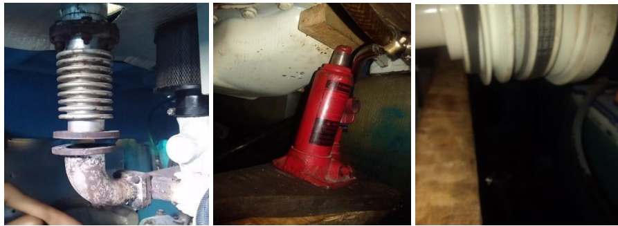
Figure 3. Adjusting the Gearbox and Main Engine Angles Relative to the Propeller Shaft
