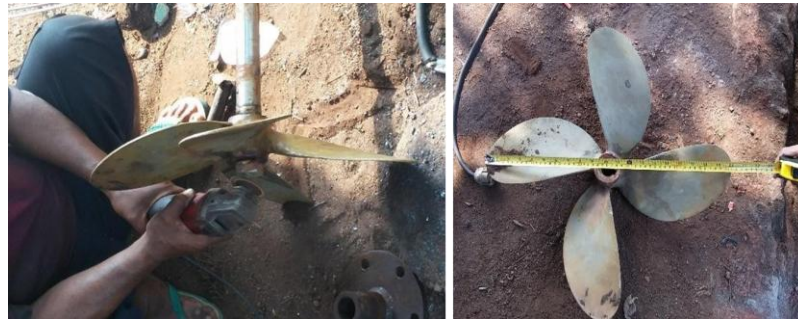
Figure 7. Replacement of D20, P18 (4 blades) with D22, P20 (3 blades)
