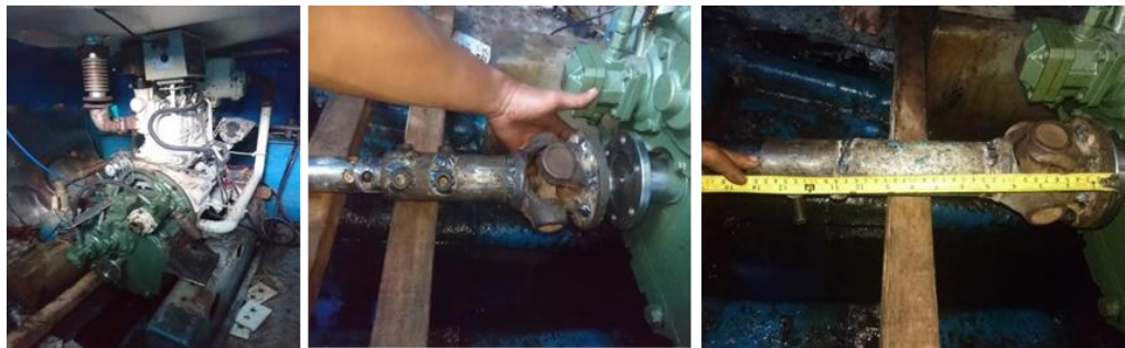
Figure 4. Universal joint installation
