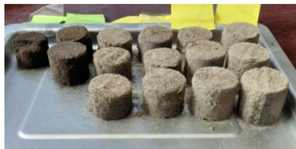
Figure 3. Peat And Gelam Wood Briquettes
