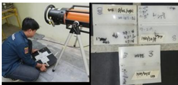
Figure 6. Radiographic NDT Testing Process
