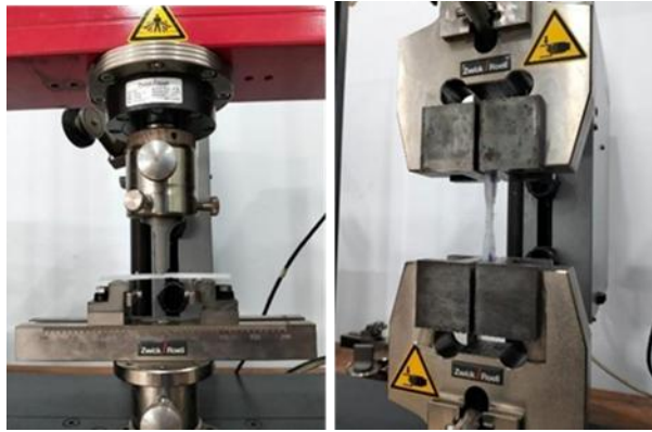
Figure 8. (a) Bending test (b) Tensile test
