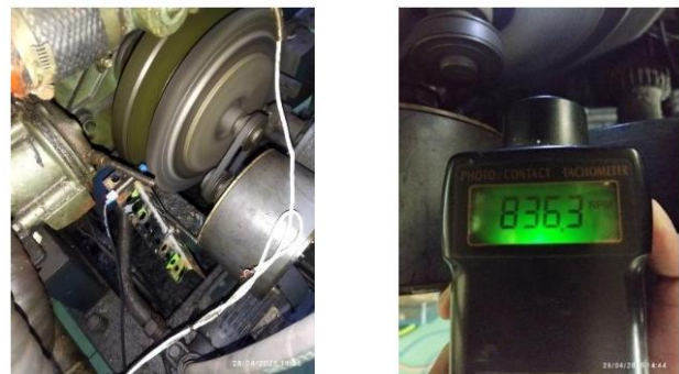
Figure 7. (a) Proximity Sensor (b) Tachometer Reading
