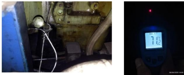
Figure 5. (a) PT100 Sensor (b) Thermogun Reading
