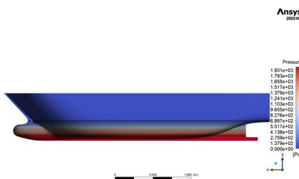
Figure 16. Pressure Contour Bare Hull, 3 kn
