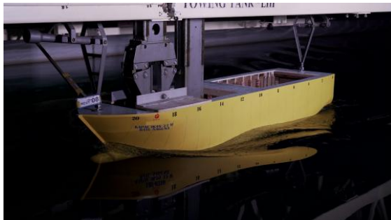
Figure 6. EFD Bare Hull, 9 kn
