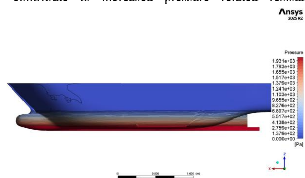
Figure 17. Pressure Contour Bilge Keel, 3 kn
