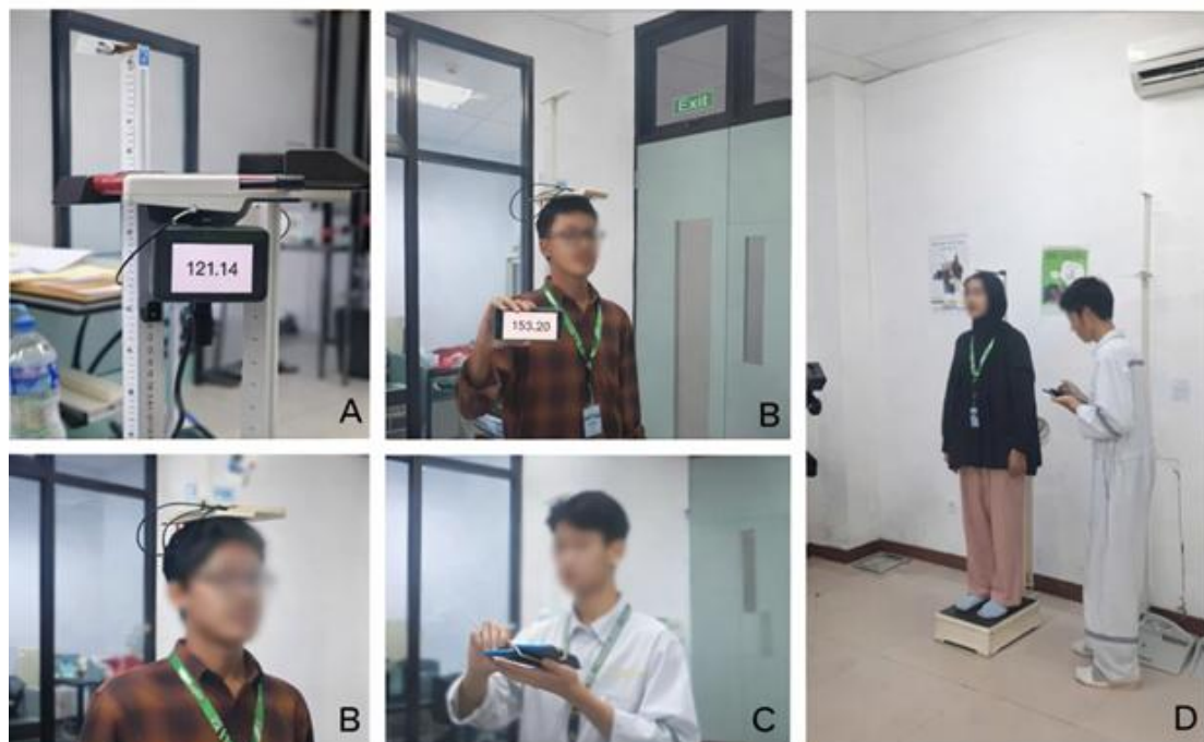
Figure 1. Digital standing-height measurement system and measurement procedures. (A) Close-up shows the sensor unit (height detector), sliding headpiece (which rests on the head), calibrated vertical frame (marked upright), and smartphone display (measured value screen). (B–C) Digital height measurement in lab tests. (D) Manual height measurement for comparison.
