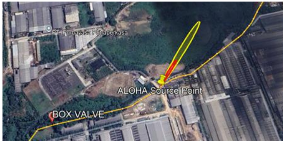
Figure 3. Downwind flammable gas dispersion under dominant wind conditions (ALOHA simulation).
