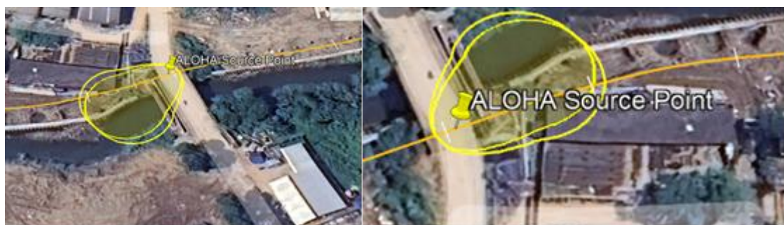
Figure 5. Comparison of VCE overpressure threat zones under calm and maximum wind conditions simulated using ALOHA.
