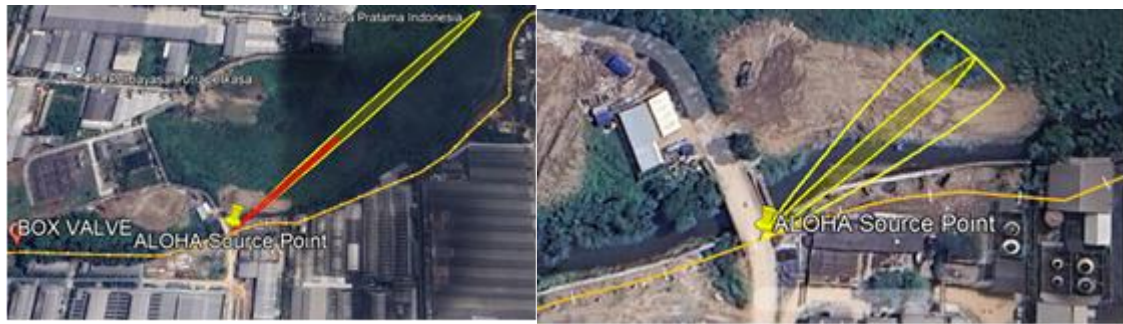
Figure 4. Downwind flammable gas dispersion footprint under maximum wind speed conditions (ALOHA simulation).
