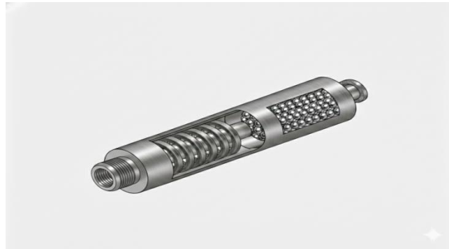
Figure 1. 3D CAD model of the hybrid PtO 2 –CeO 2 /Nd–N45 fuel catalyst device showing magnetization zone (left) and catalytic packed-bed zone (right).
