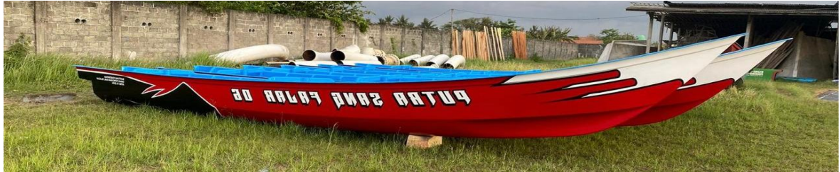
Figure 1. The boat design uses an open deck type
