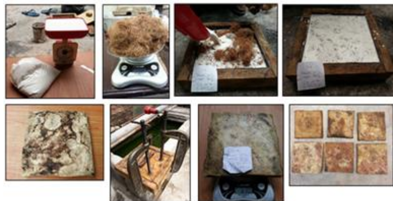
Figure 1. Stages in the Manufacturing Process of Latex–Coconut Coir Composite Specimens
