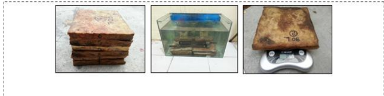
Figure 6. Measurement of Specimen Weight and Water Absorption.
