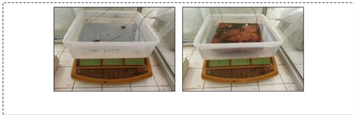
Figure 7. Illustrates the water absorption (water moisture) %
