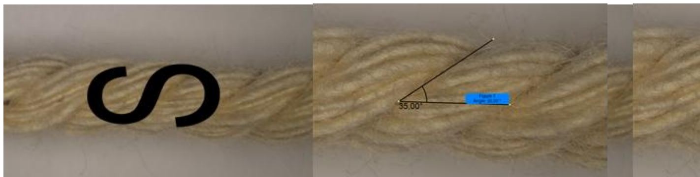
Figure 1 Twist direction and twist angle of the cotton yarn
