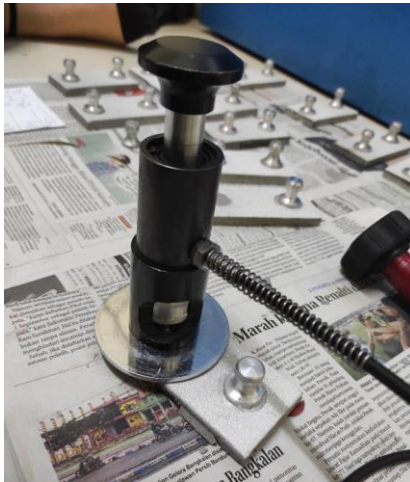
Figure 5. Pull Off Adhesion Testing Process
