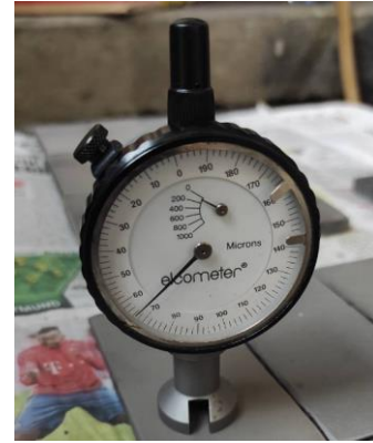
Figure 2. Surface Roughness Testing Process
