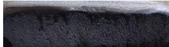
Figure 3. Coating Layer On Top of Specimen After The Coating Process
