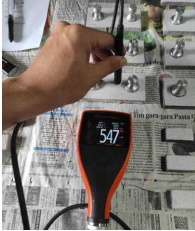
Figure 4. Dry Film Thickness Testing Process
