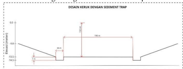
Figure 7. Sediment Trap Cross Section
