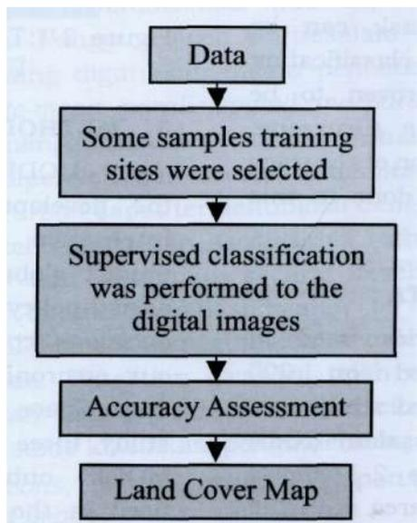
Figure 3-2: Flow chart for data processing of the images
