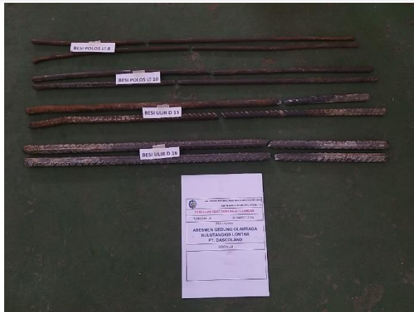
Figure 7 Reinforcement tensile test specimen
