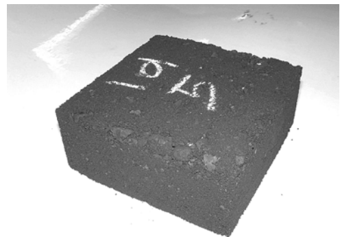
Fig. 4. The appearance of the CDWblock initially produced, with 5 percent bitumen content, with unsatisfactory coating (Mix A)
