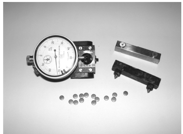
Fig. 11. A 50mm Demec gauge with its supporting equipment
