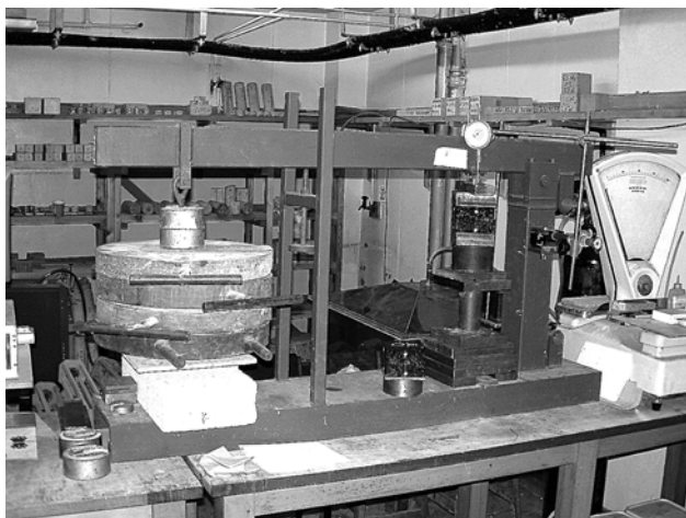
Fig. 13. Arm load machine used for creep test loading
