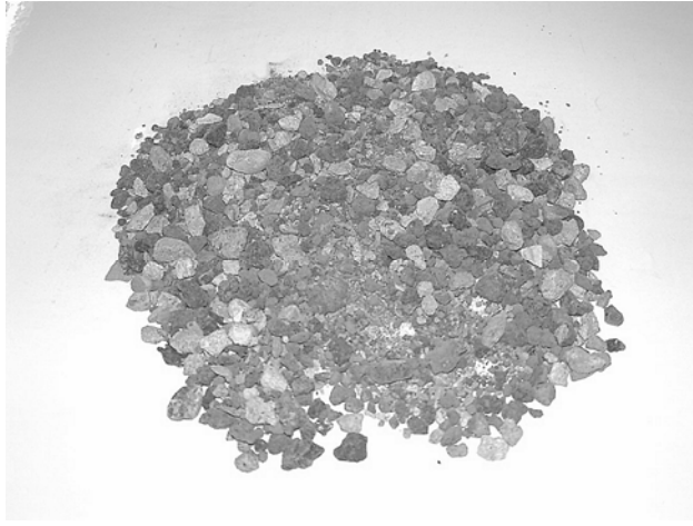
Fig. 1. The construction demolition waste (CDW) aggregate material
