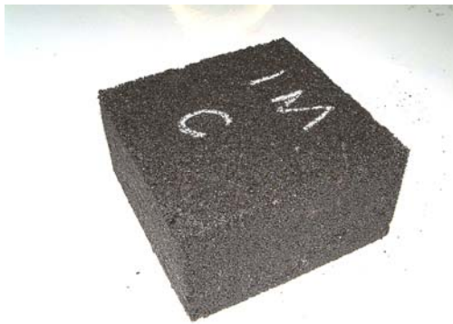
Fig. 5. The CDWblock appearance, with modified grading and with 5.5 percent bitumen content, with satisfactory coating (Mix B)
