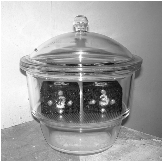
Fig. 16. Conditioning of samples in a desiccators
