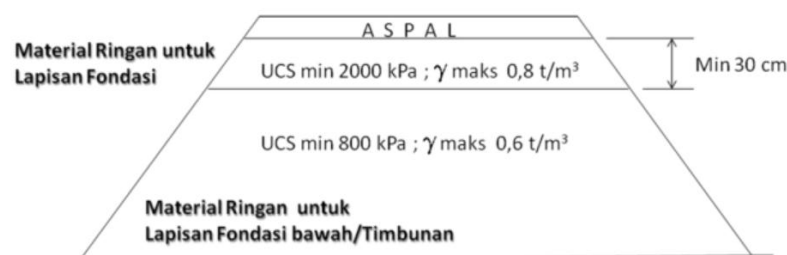
Figure 6. Typical Road Construction Using Light Foam Mortar Material
