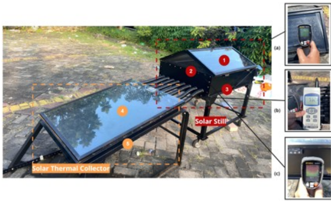
Figure 2. Measurement points of temperature in the experimental setup: (1) glass cover temperature of the solar still, (2) basin water temperature, (3) absorber plate temperature of the solar still, (4) glass cover temperature of the solar thermal collector, and (5) absorber plate temperature of the solar thermal collector.
