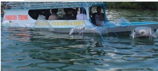
Figure 7. Sea trial of unsinkable boat
