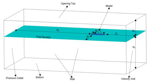
**Figure 2.** Boundary Condition Setting
