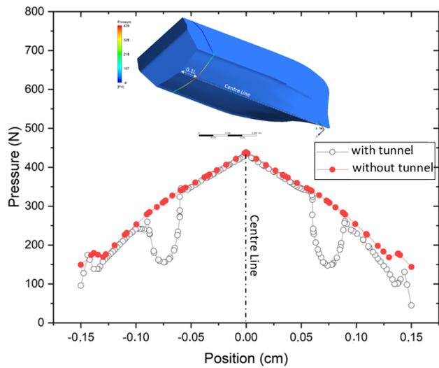
**Figure 7.** Lateral pressure distribution at 0.1L from stern of bottom at  $Fr = 0.3$
