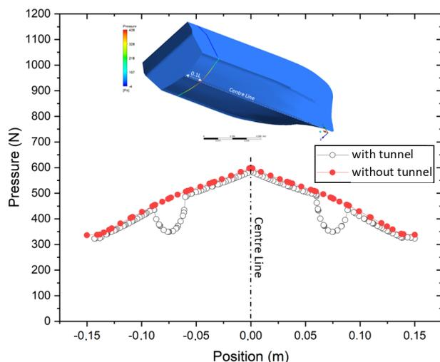
**Figure 11.** Lateral pressure distribution at 0.1L from stern of bottom at  $Fr = 0.5$
