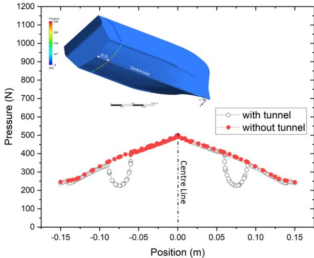
**Figure 9.** Lateral pressure distribution at 0.1L from stern of bottom at  $Fr = 0.5$
