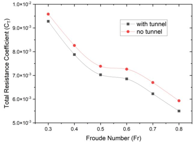
Figure 5. The differences CT at Fast Patrol Boat Models
