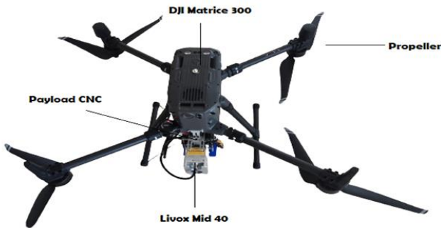
Figure 3. Payload Design on DJI M300 and LiDAR Livox
