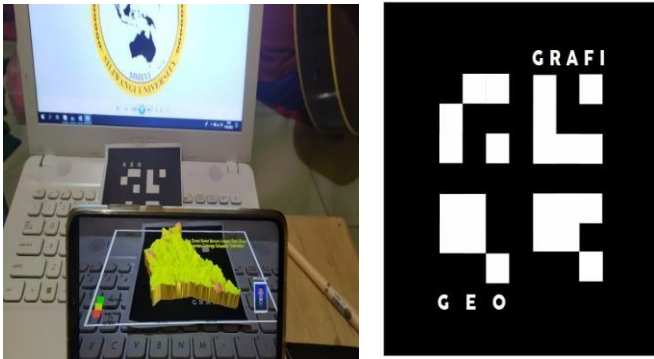
Fig. 9 View of landslide-prone 3D map and barcode scan on the Geo Camera App
