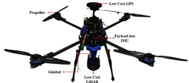
Figure 2. Low-Cost Drone LiDAR Multi-Sensor
