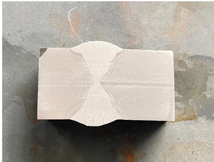
Figure 3. Macrostructure of Double V groove
