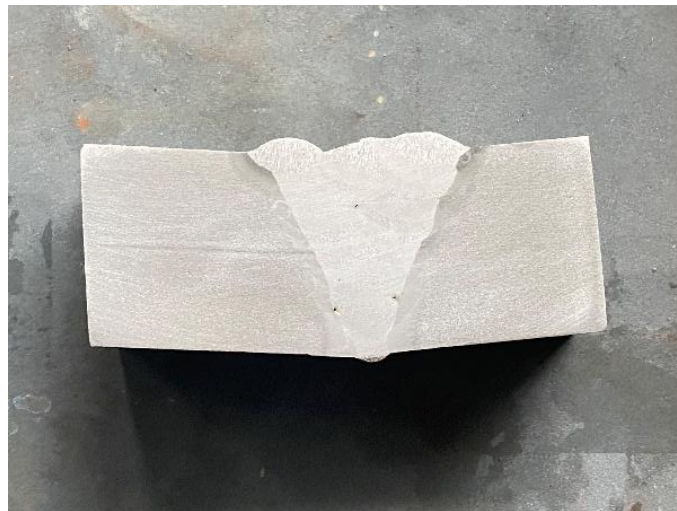
Figure 2. Macrostructure of Single V groove
