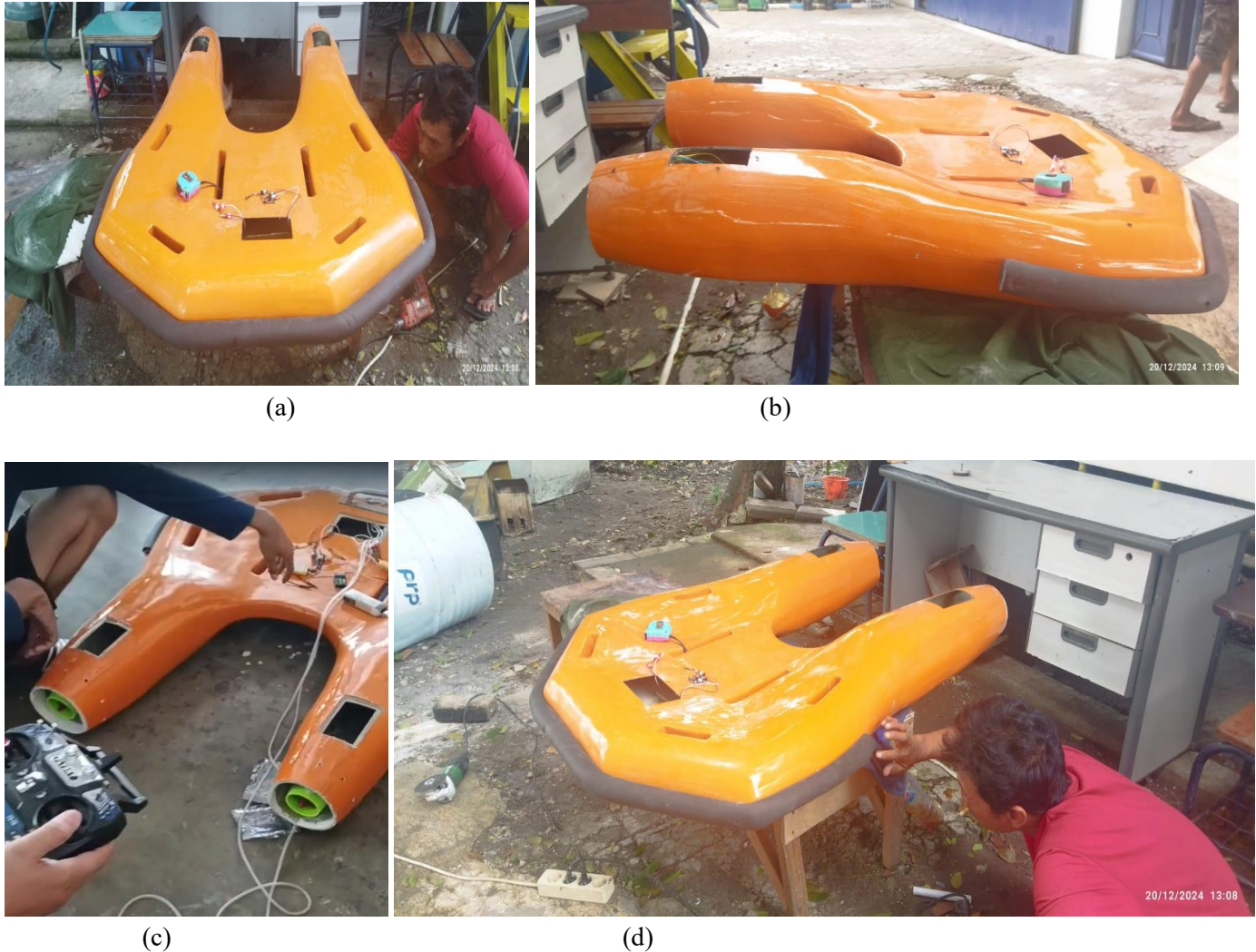
Figure 4. Product Manufacturing and Painting ((a) Body manufacturing, (b) Propulsion system installment, (c) Remote control integration, (d) Painting correction)
