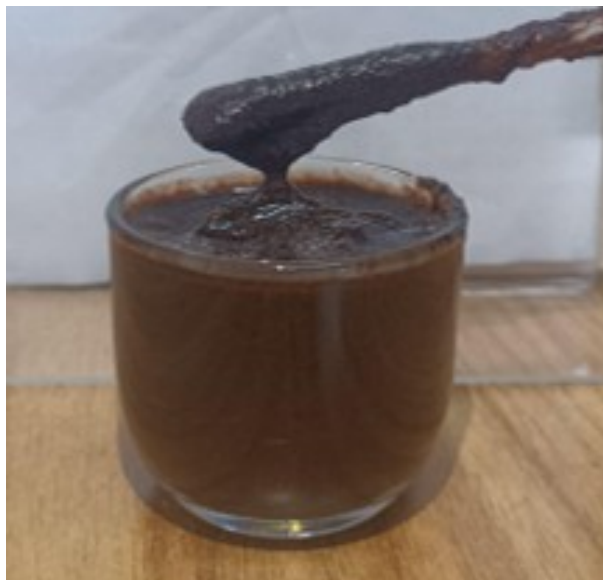
FIGURE 5 Mixture of Dextrin and Casein after Triethanolamine Addition.
