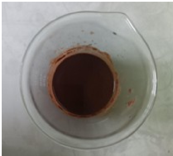
FIGURE 3 Cassava Peel Adhesive Paste after Casein Addition.
