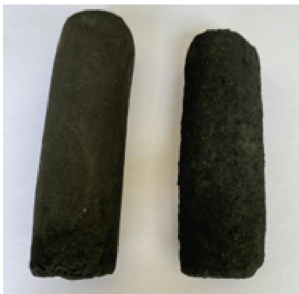
FIGURE 6 (Left) Biobriquette with Cassava Peel Binder, (Right) Commercial Biobriquette.
