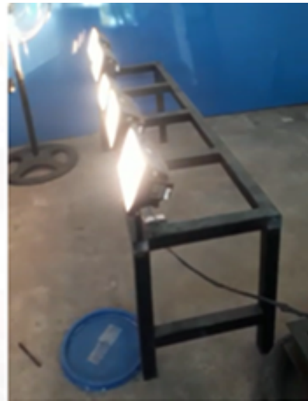
FIGURE 4 Performance Testing With Halogen Lamps
