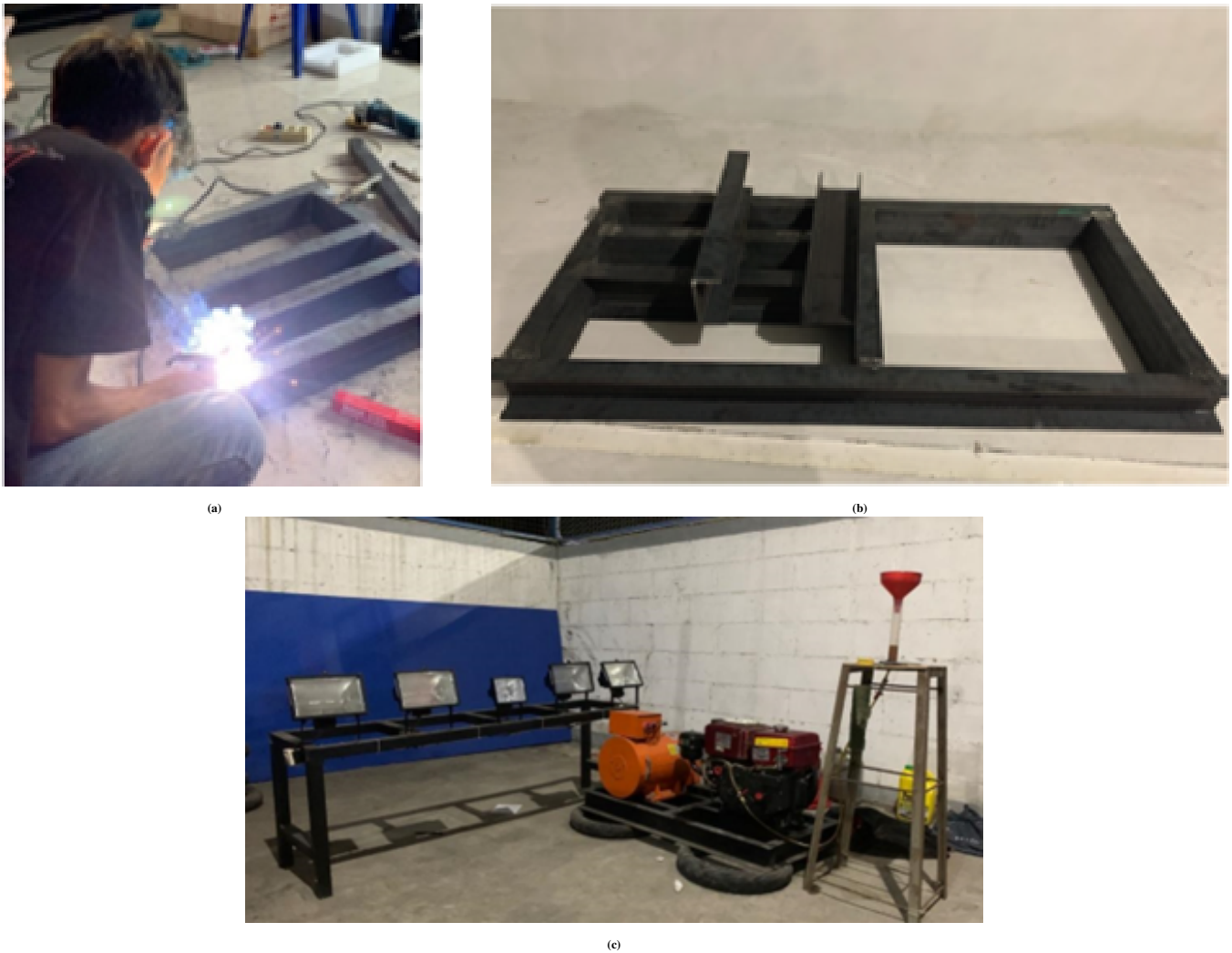
FIGURE 3 (a) Welding process for engine mount frame, (b) Engine mount frame, (c) Engine and generator are assembled to the mount frame
