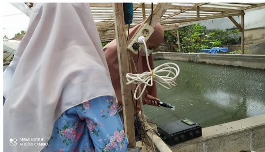
**Gambar 6** Uji coba alat sensor pH, *temperature*, dan *Dissolved Oxygen* (DO).
