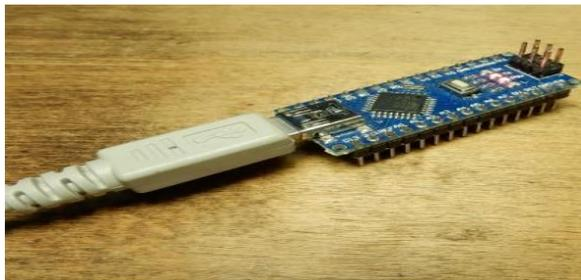
Gambar 2. Arduino to PC
