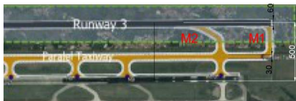
Figure 3. Measurement Results of Runway 2 and Runway 3 Separation Distance.
